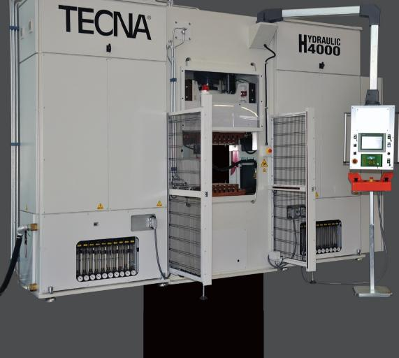
TECNA presents a new range of hydraulically operated portal welding machines
